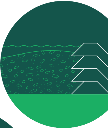
CENTERLINE In centerline dams, the dam is raised vertically from the previously constructed dam as tailings are added to the facility.
