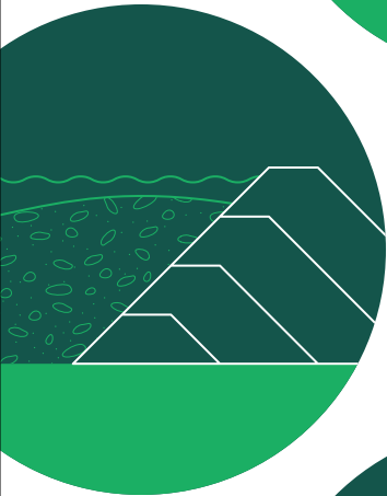
CENTERLINE In centerline dams, the dam is raised vertically from the previously constructed dam as tailings are added to the facility.
